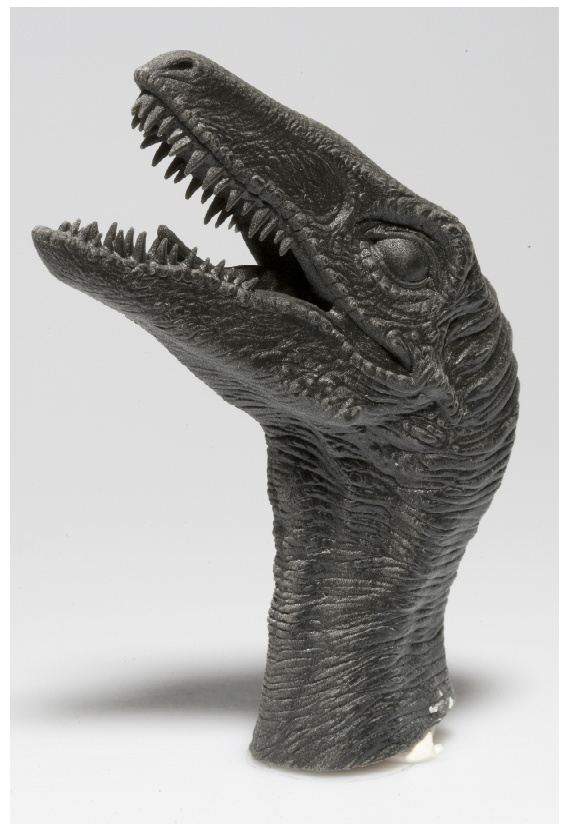
A 3D model produced using Objet's Polyjet process.
